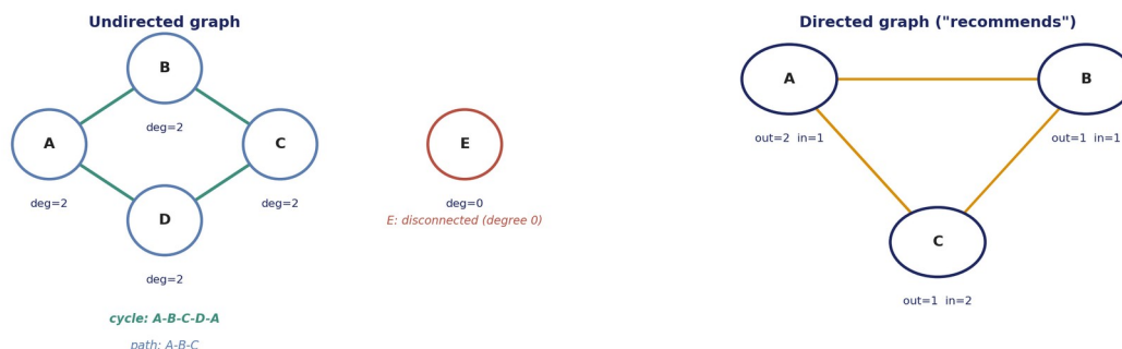
Figure 13.1 — left: an undirected 4-vertex cycle plus one disconnected vertex, with each vertex's degree labeled. Right: a small directed "recommends" graph, with in-degree and out-degree labeled separately at each vertex.
